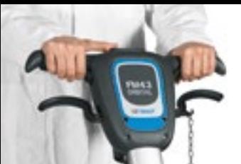
It is equipped with a safety system through which the machine activation depends on the simultaneous pressure of the handlebars levers and dead's man button. When the levers are released the machine stops
