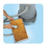
It is important to clean the panel filter with a vacuum cleaner after each cleaning task in order to guarantee perfect machine performance
