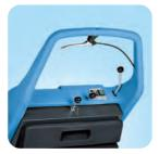
Controls: Suction on/off control, mechanic filter shaker, side brush lifting/lowering mechanism, traction control (on the traction models)
