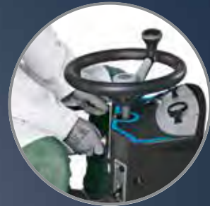
The brushes (central and side) are easily moved with the aid of 2 levers
