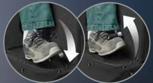
Pedal controls for forward/backward direction
